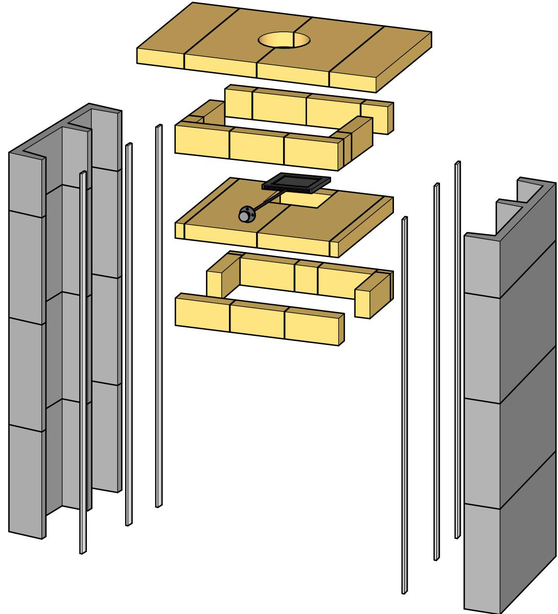
The 5-Run Heat Exchanger is a compact top-venting heat exchange strategy. It is called the 5-Run because the gases first go upwards from the firebox. We recommend a bypass damper be installed. When open, the flue gases have an easy path to prime the chimney and establish draft. When closed, the gases split into two symmetric downdrafts. In the base, they turn around and become two symmetric updrafts before collecting in the chimney. These five flues give the name 5-Run to this configuration.
