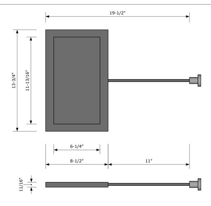
Bypass Damper Installation Instructions: https://www.firespeaking.com/how-to/bypass-damper-installation
